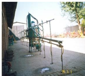
Drop pipe boom sprayer Source: www.uaf.edu.pk GOP Patent No. 139290
