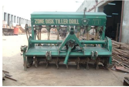
Zone disk tillage machine (GOP Patent 139296) developed at UAF
