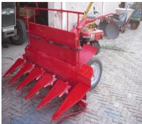
Indigenized Self-propelled multi-crop reaper, Source; www.uaf.edu.pk
