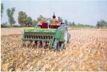
Zero tillage machine developed at FMI, PARC, Islamabad (Source: Raza et al. 2006)
